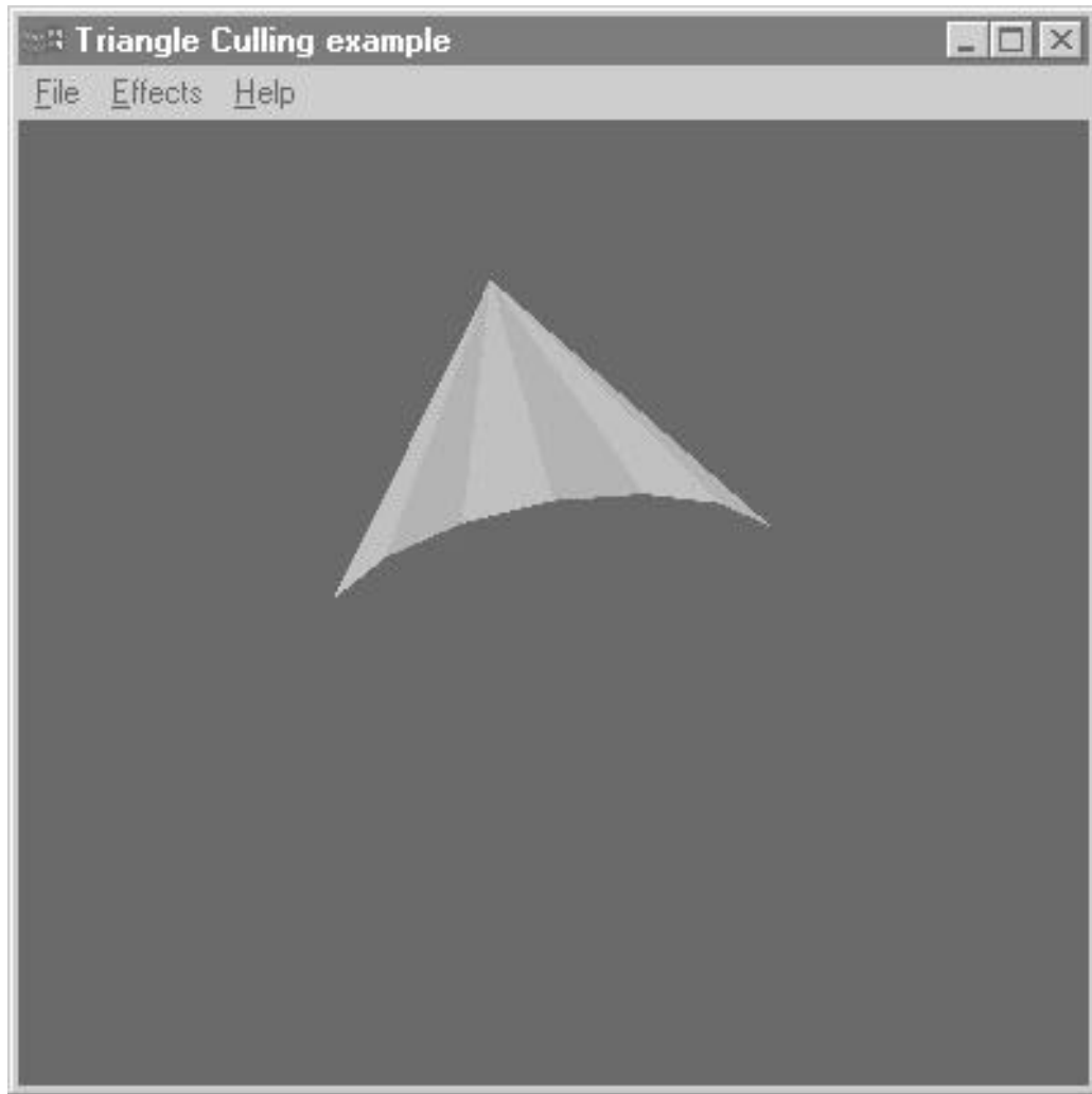
Figure 6-20 The bottom of the cone is culled because the front-facing triangles are inside
