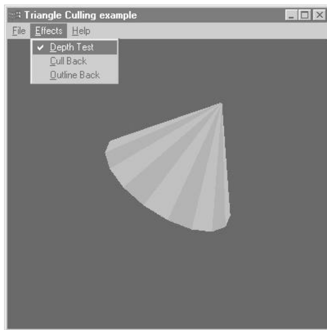
Figure 6-18 The bottom of the cone is now correctly placed behind the sides for this orientation
